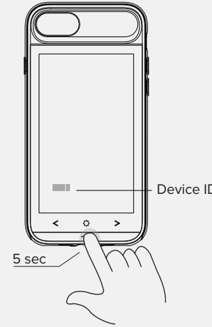
Press and hold the Power Button for 5 seconds, to switch on the InkCase i7.
